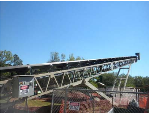
100' Long Conveyor and Hydraulic Drive for Raising and Lowering
